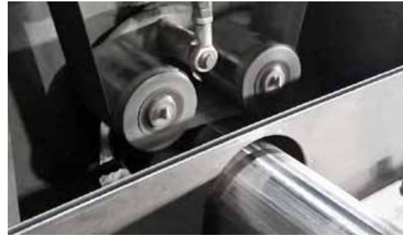
Grinding of longitudinally welded tubes
