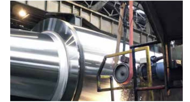
Cylindrical grinding of rollers during roller pass
