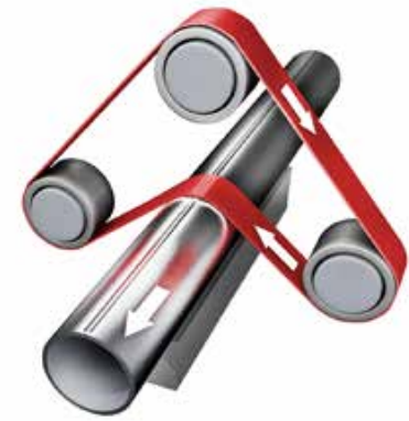
Grinding of longitudinally welded tubes
