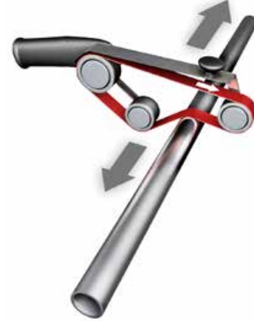
Cylindrical grinding of tubes and bars using hand-held machines
