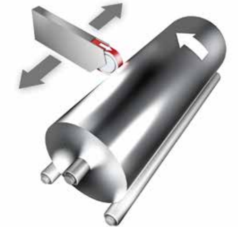
Cylindrical grinding of rollers during roller pass
