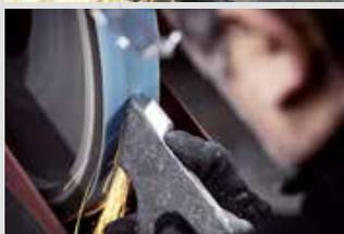
Grinding of cast parts
