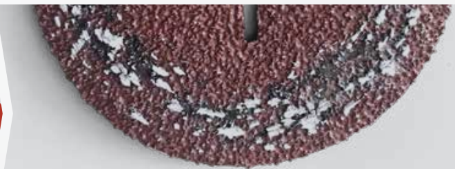
Fibre disc clogged with aluminium chips
