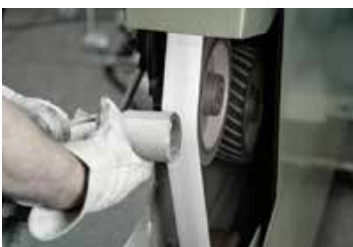
Grinding of cast parts
