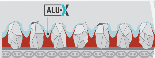
The VSM ALU-X additional layer significantly reduces adhesion; the abrasive can be used for longer.
