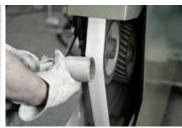
**Grinding of cast parts**
