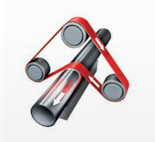
Grinding of longitudinally welded tubes
