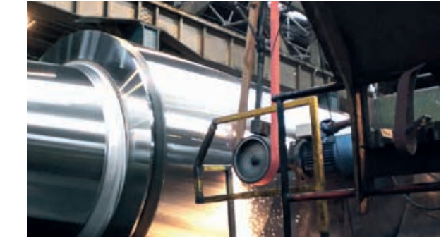
Cylindrical grinding of rollers during roller pass
