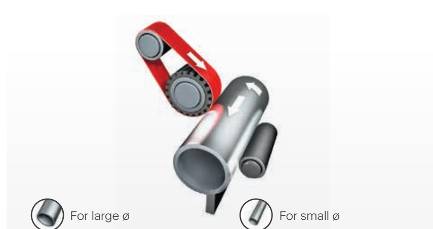
Centerless grinding of tubes and bars
