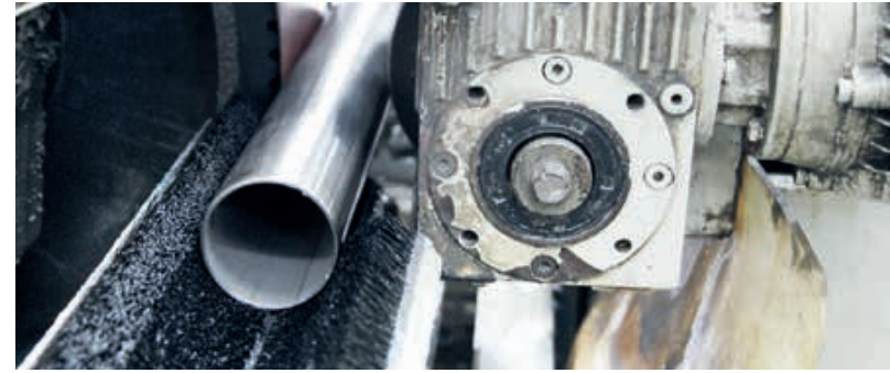
Centerless grinding of tubes and bars
