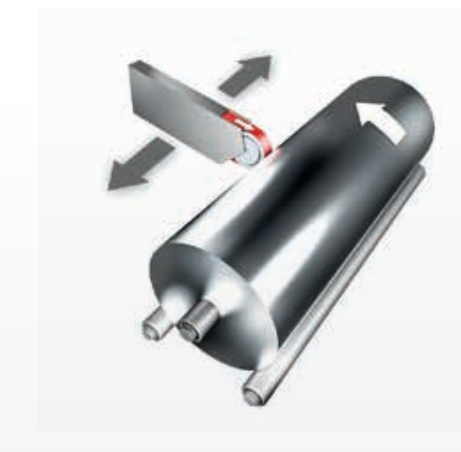
Cylindrical grinding of rollers during roller pass
