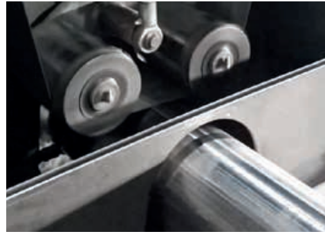
Grinding of longitudinally welded tubes
