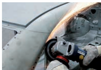
Levelling of welding seams
