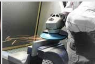
Weld seam preparation
