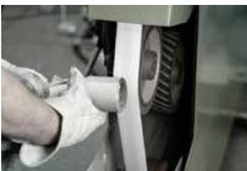
Grinding of cast parts
