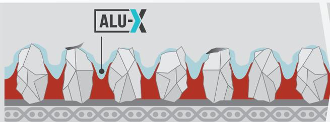
The VSM ALU-X additional layer significantly reduces adhesion; the abrasive can be used for longer.
