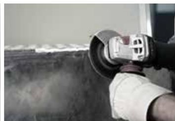
Removing welded seams
