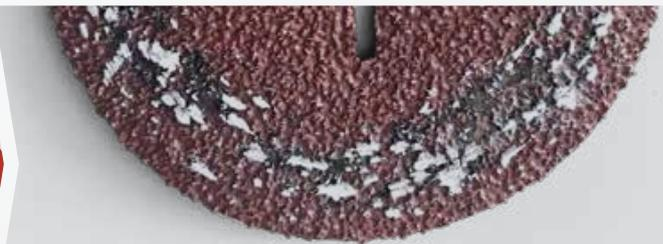
Fibre disc clogged with aluminium chips
