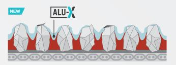
**VSM ALU-X** significantly reduces chip adhesion when processing non-ferrous metals and thus also reduces clogging of the abrasive. The service life is assured and extended so dramatically that excellent stock removal is achieved even after longer periods of use.
