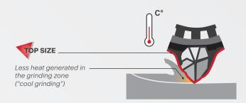
**VSM TOP SIZE** is recommended for dry machining heat-resistant stainless steels and non-ferrous metals. The grinding-active additional layer improves the cutting performance whilst reducing the temperature in the contact zone. This significantly extends the service life of the abrasive.
