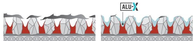
*Conventional abrasives: Chips stick to the grain tips and the abrasive becomes clogged.*
